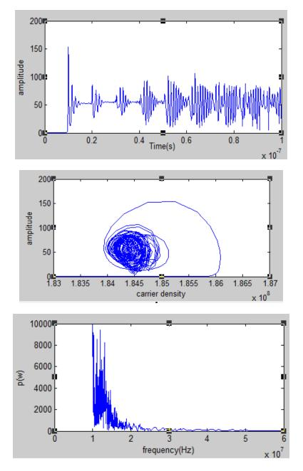
Fig. 6 time series of the laser output power, its phase portrait and corresponding FFT spectrum. at k=  $36e^{-1} ns^{-1}$ ,  $i_{dc} = 10mA$ ,  $i_{ac} = 5mA$ ,  $f_m = 100e^6$  Hz.
