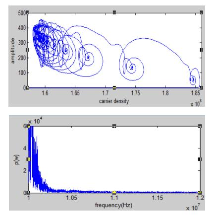
Fig. 9time series of the laser output power, its phase portrait and corresponding FFT spectrum. at k= 360 ns<sup>-1</sup>,  $i_{dc} = 10\text{mA}$ ,  $i_{ac} = 5\text{mA}$ ,  $f_m = 100\text{e}^6$  Hz.
