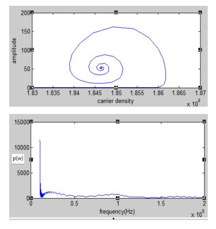
Fig. 4 time series of the laser output power, its phase portrait and corresponding FFT spectrum. at k=  $36e^{-4} \text{ ns}^{-1}$ ,  $i_{dc} = 10\text{mA}$ ,  $i_{ac} = 5\text{mA}$ ,  $f_m = 100e^6$  Hz.
