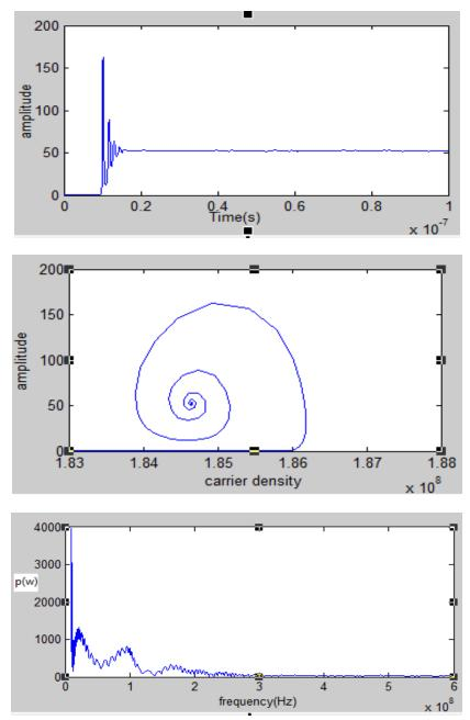
Fig. 2 time series of the laser output power, its phase portrait and corresponding FFT spectrum. at k= 36e<sup>-8</sup>ns<sup>-1</sup>,  $i_{ac} = 10$ mA ,  $i_{ac} = 5$ mA,  $f_m = 100e^6$  Hz.
