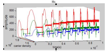
Fig. 13 phase portrait for amplitude versus carrier density and time. at k= 360 ns<sup>-1</sup>,  $i_{dc} = 10$ mA ,  $i_{ac} = 5$ mA,  $f_m = 100e^6$  Hz.
