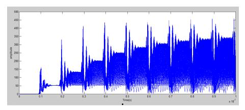
Fig. 11 time series of the laser amplitude.at k= 360 ns<sup>-1</sup>,  $i_{dc}$  =10mA ,  $i_{ac}$  = 5mA,  $f_m$  = 100e<sup>6</sup> Hz.
