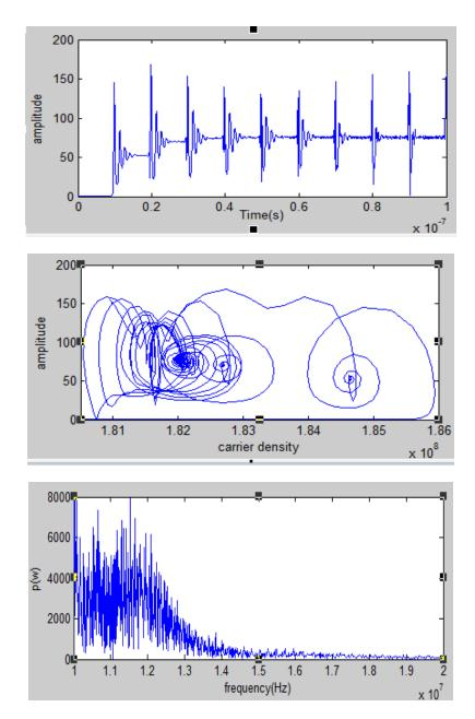
Fig. 8 time series of the laser output power, its phase portrait and corresponding FFT spectrum. at k= 36 ns<sup>-1</sup>,  $i_{dc}$  =10mA ,  $i_{ac}$  = 5mA,  $f_m$  = 100e<sup>6</sup> Hz.
