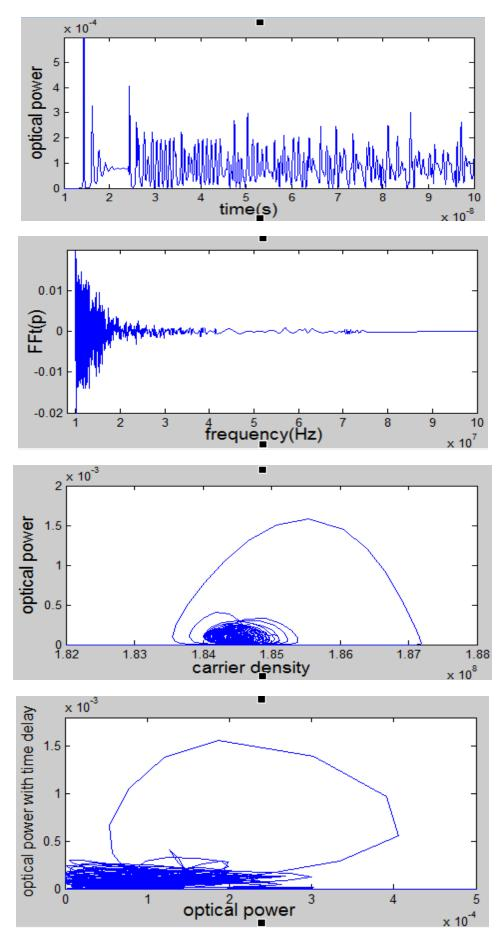
Fig. 7 The time series of the laser output power, its corresponding FFT spectrum and phase portrait. At k=  $36e^{-1}ns^{-1}$ ,  $i_{ac} = 10mA$ ,  $i_{ac} = 5mA$ ,  $f_m = 100e^6$  Hz.
