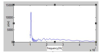
Fig. 5 time series of the laser output power, its phase portrait and corresponding FFT spectrum. at k=  $36e^{-2} ns^{-1}$ ,  $i_{dc} = 10mA$ ,  $i_{ac} = 5mA$ ,  $f_m = 100e^6$  Hz.
